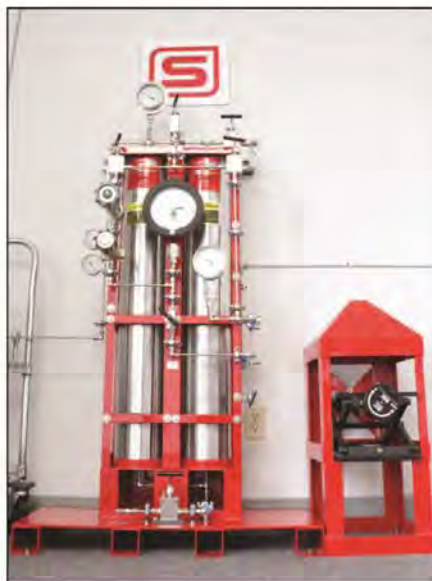
High-Pressure Accumulator Tank and Burst Test Manifold
