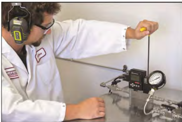
Mass Flow Controller Calibration: Valve Adjustment
