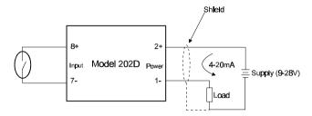
Connection to a Sensor requiring External Power
