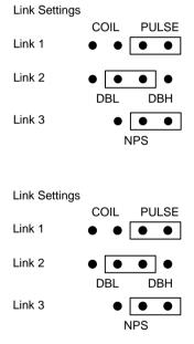
eg. Positive displacement flowmeters with reed switch outputs.
