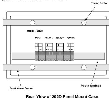
A diagram of the rear panel is shown below:
