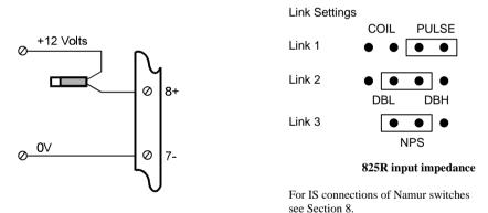
Note: Use this connection for battery or loop powered versions of the Model 202D. If a 4-20mA output is installed, the supply to the proximity switch must be isolated.
