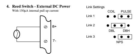
Note: For a switch or reed input with contact bounce link DBH can be switched "on". This will eliminate the effect of switch bounce while limiting the input frequency to 200Hz.
