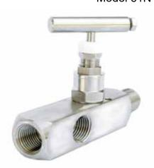
All units with a male process connection can also be supplied with either a standard or extended weldable connection. All units incorporate the Budenberg Needle Valve Head assemblythat is suitable for operating pressures up to 10,000 psig and temperatures up to 450°c in conformance to ASME / ANSIB16.34 Class 2500. Available in a full range of materials, configurations, connections options, ensure that there is a model for virtually any application or environment.
