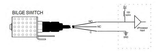
For higher voltages, resistors in series provide a voltage change across the input whilst maintaining a sufficiently high current through the switch contacts.
