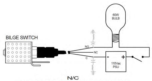
Connect negative (-) to the bilge switch common lead & positive to the bilge switch N/C lead. In an upright position the lamp should be on, lift the test handle & the lamp should go off.
