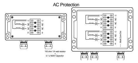
Suitable arc suppression components are supplied loose with the PSM junction boxes.
