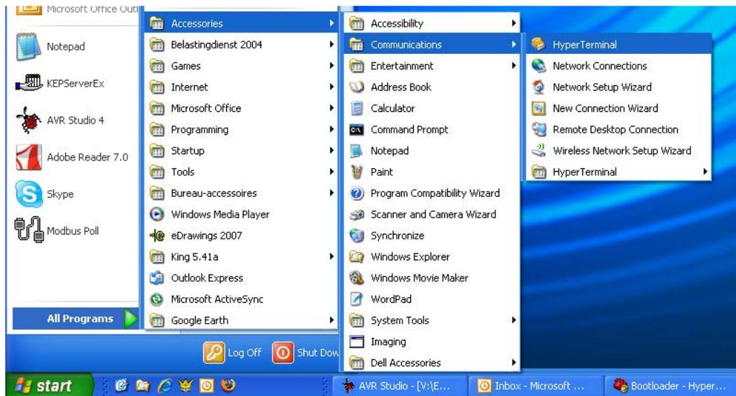
Start HyperTerminal from windows and select the com port to which the RS485 interface is connected. Use the following settings:
