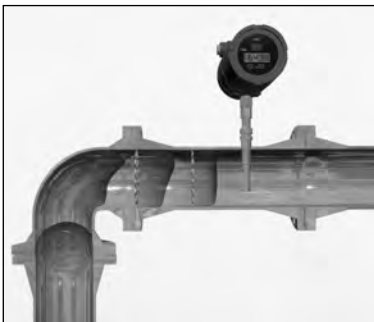
Built-in flow conditioning creates a uniform velocity profile in constrained applications
