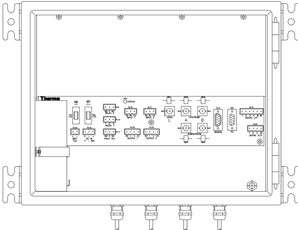
**Fig 2 Sarasota 200 with lid open showing internal components**
