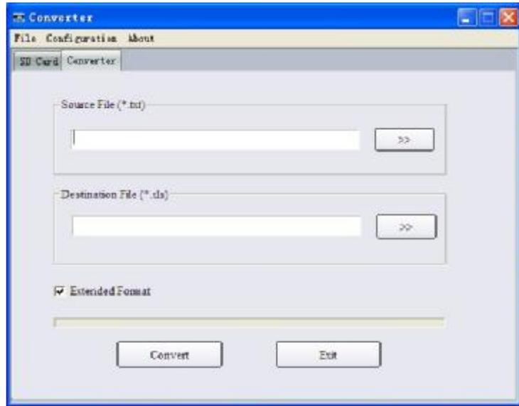
Select the file to be converted in “Source File (\*.txt), enter the directory path and the filename in “Destination File (\*.xls), then press “Convert”. The conversion is completed.
