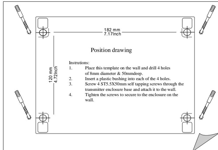
Take out the enclosed screws and plastic bushings. Insert the plastic bushings into the installing holes. Then open the two aluminum pieces on the two sides of the top cover. Put the flowmeter into the position and screw it in. (right picture)
