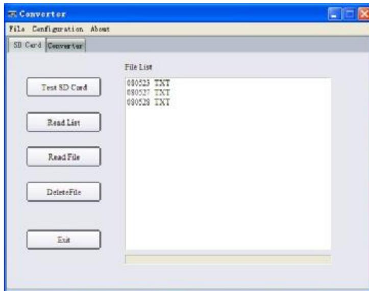
After the reading, will pop up "The File has been read" window and Converter.exe the root directory of storage or set up by reading the paper and check the contents of the file format is normal.
