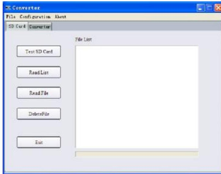
Due to the expanded memory (EMS) capacity of the flowmeter is extremely small as compared with the SD memory card; the transfer speed is rather slow for some commands. So we suggest: it is better to read the SD data externally (remove the card from the flowmeter to insert it into your PC).
