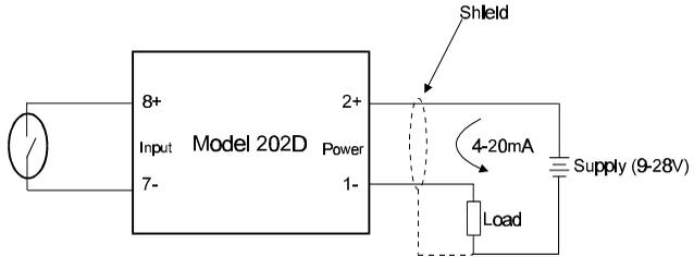
**Connection to a Sensor requiring External Power**
