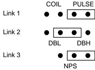
Note: For a switch or reed input with contact bounce link DBH can be switched "on". This will eliminate the effect of switch bounce while limiting the input frequency to 200Hz.
