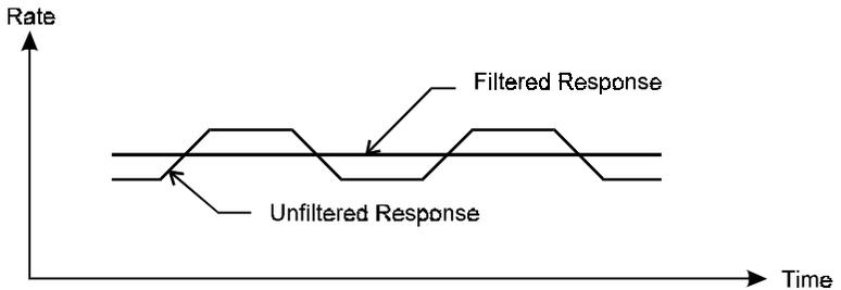
As a guideline to the degree of filtering to be used, the following table shows the response to a step change in input. The value, CAL 06, is the filter constant which is programmed during the Programming routine. The times for the display value to reach 90% and 99% of full swing are given in seconds, for different values of CAL 06.
