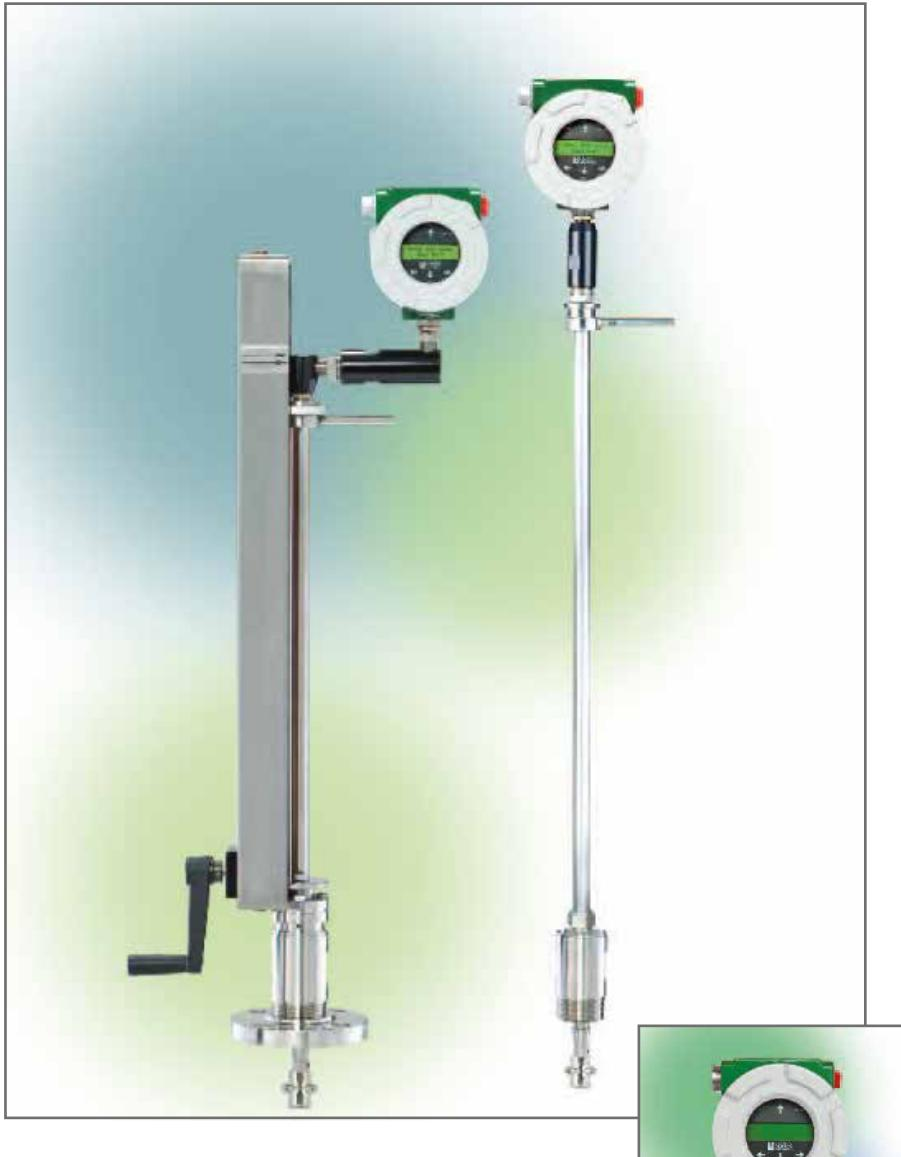
Vortek Instruments' Pro-V multivariable flowmeters utilise three primary sensing elements - a vortex shedding velocity sensor, an RTD temperature sensor and a solid-state pressure transducer - to measure the mass flow rate of gases, liquid and steam.
